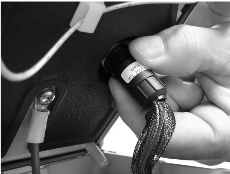
Figure 11-3: Wire Harness Disconnection
