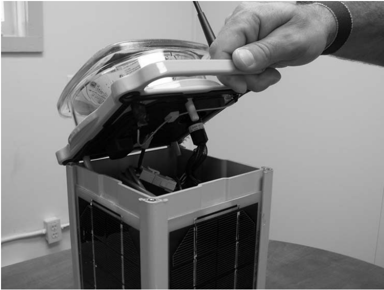
Figure 11-2: Lifting off the Head
