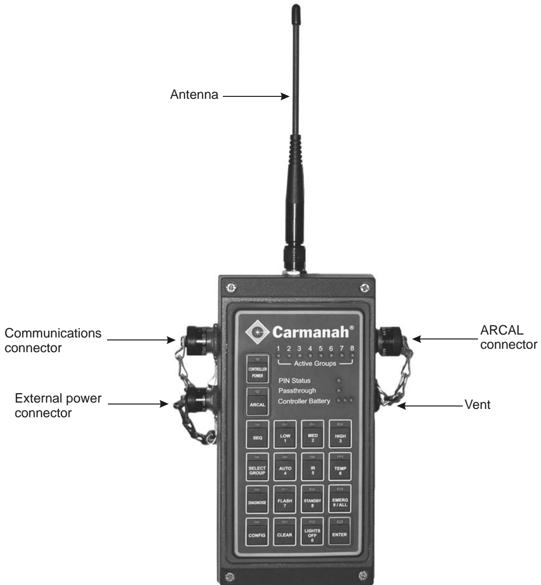
Figure 3-2: Wireless Controller Component Identification
