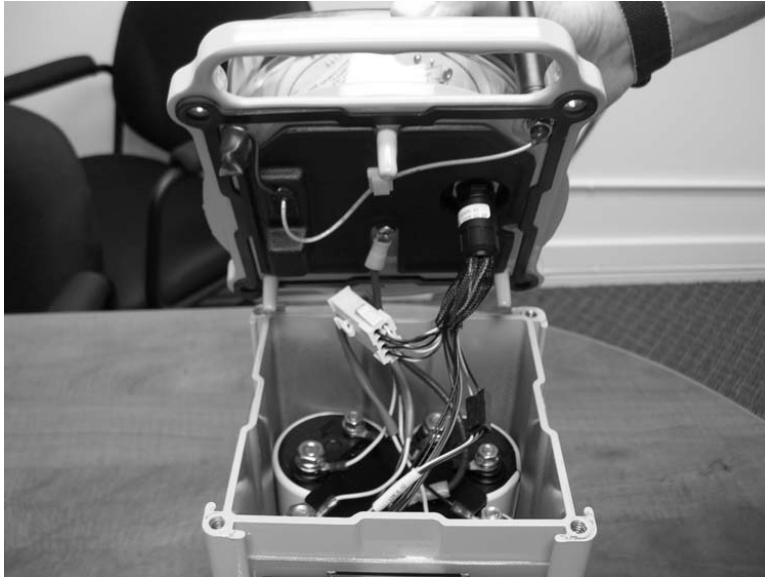
Figure 11-12: Replacing the Head
