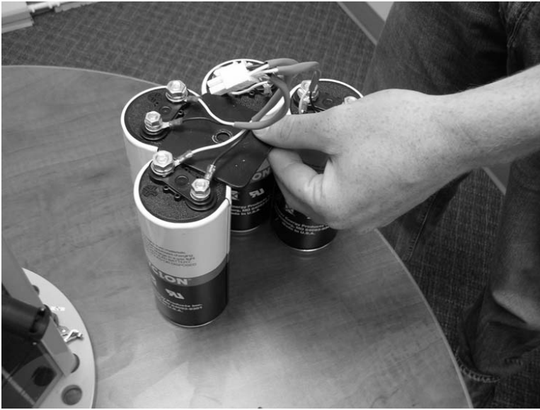
Figure 11-8: Removing the Battery Top Plate
