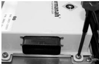
Figure 6-2: Removing EMS fasteners
